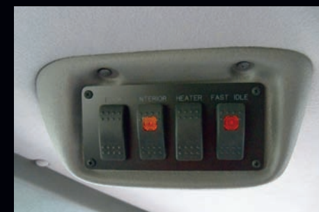
Conveniently located switch panel on driver's overhead
